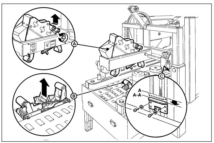
Figure 6-3 – Removing Taping Heads from Case Sealer 34
